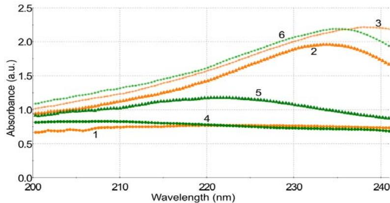
Figure 9. The gamma-ray induced optical absorption for: 1 – non-irradiated OFS2 (600  $\mu\text{m}$  core diameter); 2 – OFS2 (600  $\mu\text{m}$  core diameter) total irradiation dose of 3 kGy; 3 – OFS2 (600  $\mu\text{m}$  core diameter) total irradiation dose of 13 kGy; 4 – non-irradiated OFS2 (1000  $\mu\text{m}$  core diameter); 5 – OFS2 (1000  $\mu\text{m}$  core diameter) total irradiation dose of 3 kGy; 6 – OFS2 (1000  $\mu\text{m}$  core diameter) total irradiation dose of 13 kGy.
