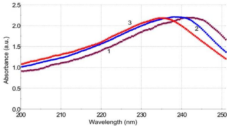
Figure 8. The gamma-ray induced optical absorption at the total irradiation dose of 10 kGy for: 1 – OFS2 (400  $\mu\text{m}$  core diameter); 2 – OFS2 (600  $\mu\text{m}$  core diameter); 3 – OFS2 (1000  $\mu\text{m}$  core diameter).
