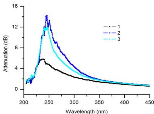
Figure 2. The radiation induced change in the optical absorption of the sample in the first hour of irradiation: 1 – the un-irradiated sample; 2 – at 0.33 kGy total irradiation dose; 3 – the optical transmission recovery after the sample was kept non-irradiated for about 18 hours.
