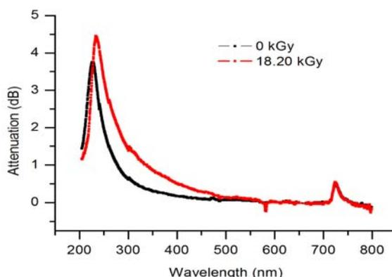
Figure 6. The optical absorption of the two optical fibers probes (each of 6 m length)
