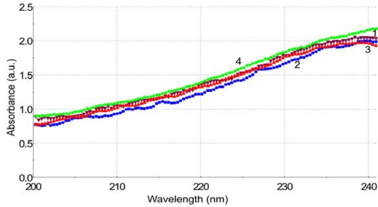
Figure 7. The gamma-ray induced optical absorption at the total irradiation dose of 10 kGy for: 1 – OFS1 (400  $\mu\text{m}$  core diameter, black Tefzel jacket); 2 – OFS1 (400  $\mu\text{m}$  core diameter, Polyimide jacket); 3 – OFS1 (400  $\mu\text{m}$  core diameter, Tefzel jacket); 4 – OFS2 (400  $\mu\text{m}$  core diameter, Tefzel jacket from a second manufacturer).
