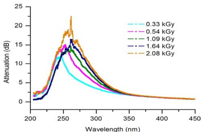
Figure 3. The dependence of the optical absorption on the total irradiation dose, for the first 10 hours of irradiation.
