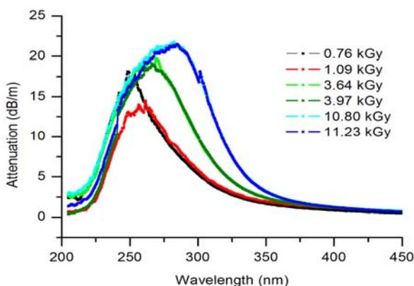
Figure 5. The effect of the optical irradiation of the sample during gamma-ray irradiation.
