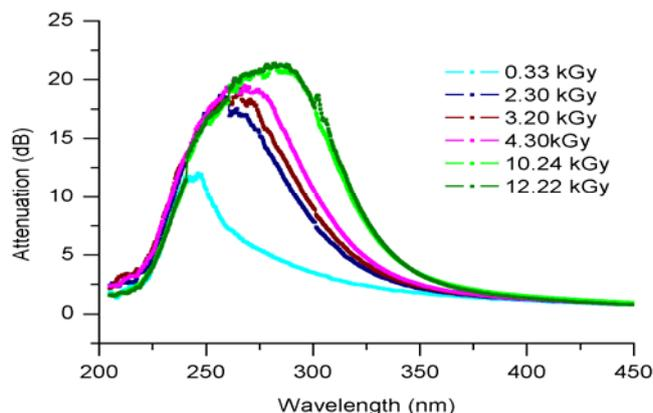
Figure 4. The dependence of the optical absorption on the total irradiation dose, for the first 3 days of irradiation.
